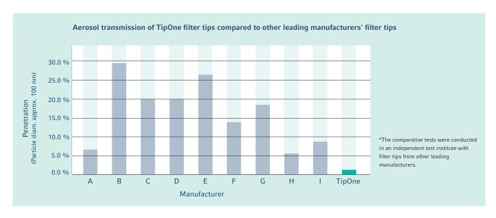
In this investigation TipOne® 200  $\mu$ l filter tips have been compared with those of nine other leading manufacturers by testing the blocking efficiency of filter tips using airborne particles. The results of this test shows the TipOne® filter can effectively block more than 99% aerosols.
