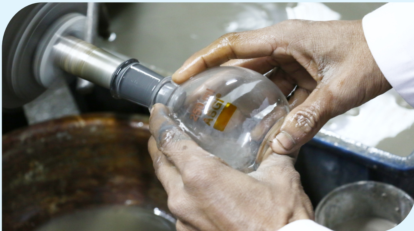
grinding & polishing of joints
