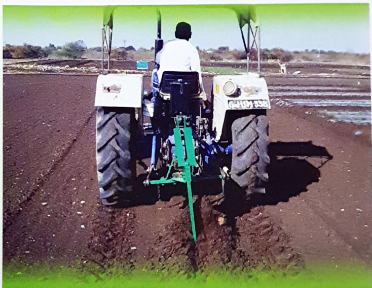
Figure 7: Sub-soiling for improving rain water infiltration.
